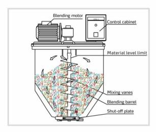
Signals from the control cabinet will be sent to blending motor which drives the blending screw to start material blending. Then material conveyed along the cylinder up to the top is evenly spread in the blending barrel. This process mixes material evenly in a short time, saving energy. After blending, draw open the shut-off plate to discharge the material.
